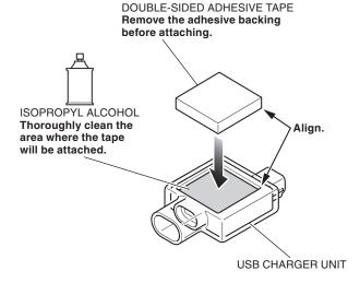
6. Install the USB charger unit as shown.
